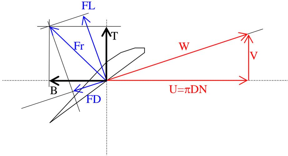
The blade is moving tangentially with a velocity  $U$  and axially with a velocity  $V$ . An aerodynamic force  $F_r$  is thus created on the blade. This force could be decomposed into a thrust  $T$  and braking force  $B$ . The blade input power is then a product of the tangential velocity and the braking force while the blade useful power is the product of the thrust and the axial velocity.
